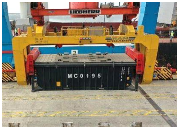
Copper concentrate in flip containers being loaded by rotating spreader Revolver at TPS Valparaíso.
