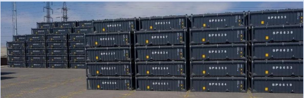
A containerised system uses up the storage capacity per square meter, as the commodity is stored in a cuboid formation rather than a conical or cone formation (shown below)
